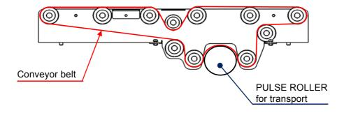
[How to Replace a PULSE ROLLER for transport] (See Fig. 6)
